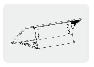
Open the angle locks. Slowly put down the solar panel and make the angle locks slip into the right angle. Then tighten the angle locks again.
