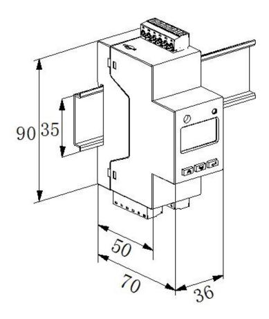
Fix the DTU onto the rails of AC distribution box. Connect the L and N cable to port 11 and port 14. Then connect CT cable to port 4 and port 5.
