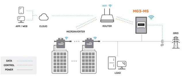
The microinverter converts the DC electricity generated by solar panels into AC electricity which is in accordance with the requirements of the public grid and sends the AC into the grid, reducing the load pressure of the grid.
